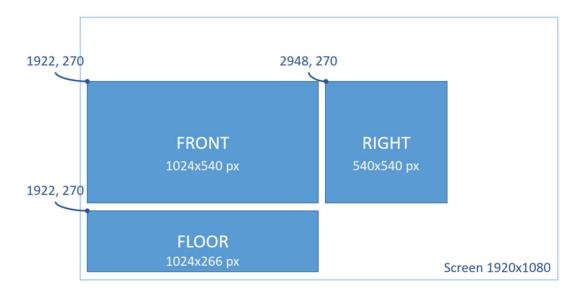
The picture above shows the resolution and desktop offset in pixel for each window. Please note, that the resolution aspect ratio needs to match the physical dimensions, i.e. if your wall is 2000x1000mm, your resolution needs to have an aspect ratio of 2:1 (like 2048x1024).
