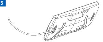
Bend flexible hosing to position that will allow webcam to have clear view of user's hand and screen.
