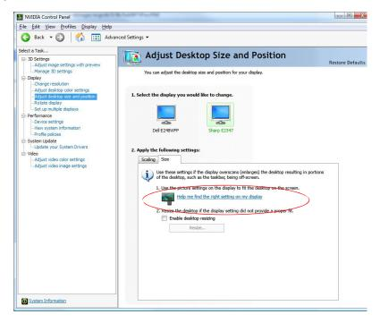
The resize controls on the NVIDIA Control Panel are provided in case satisfactory results cannot be achieved using the controls on the display.
