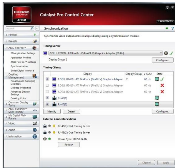
Figure 2: TimingServer using external HouseSync
