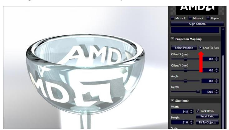
If you want to prevent the decal from projecting through the glass, select the face by toggling the Face button and clicking the surface to apply the decal.
