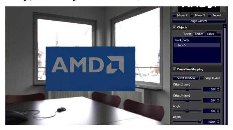
Enable the **Select Position** toggle, and slightly adjust the **Offset X** and **Offset Y** (The X and Y axis are relative to the decal).
