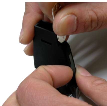
BATTERY TOOL to unlock the battery
