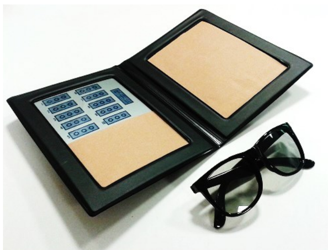
Figure 3-10. Randot™ ('Random Dot') Stereo Test (Stereo Optical Co., 2009). The 'Circles (with random dot ground)' test, was carried out by each participant to determine their stereoacuity. 10/10 correct answers = 400 seconds of arc. As shown in the image, the other tests were obscured by cardboard. Image author's own.
