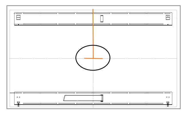
2 Draw a short (about 1") horizontal line and then a vertical line to just below the top edge of the display.
