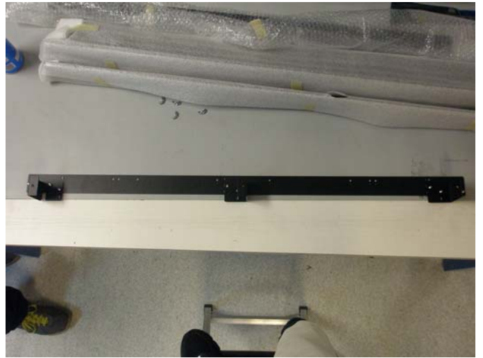
Mount bracket offset forward for use with LX46HDS, LX55HDS, and MX55HDX panels
