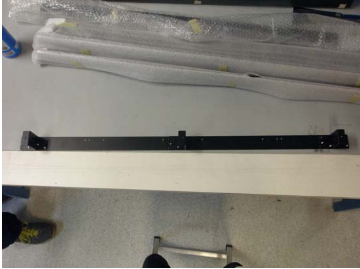
Mount bracket placement on a long bar for the top of a 55 HDU
