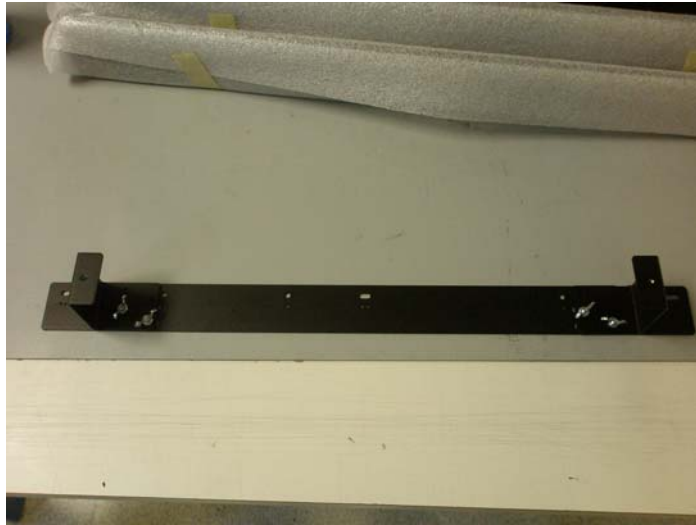
Mount bracket placement on a short bar
