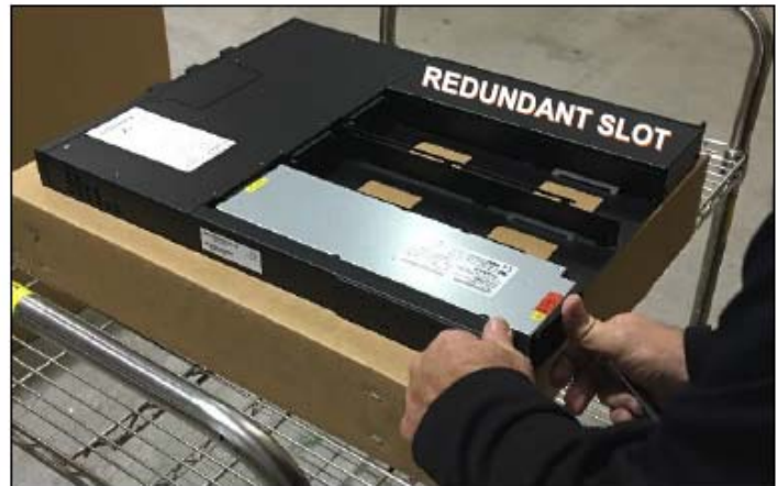
Example of RPS with three RPSM slots. Open slots vary with order
