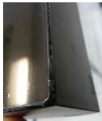
Silicone pulling out of seams (ERO units only)
