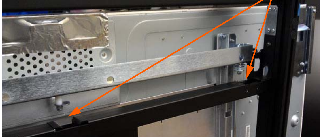
Landscape installation - Slide down and into position
