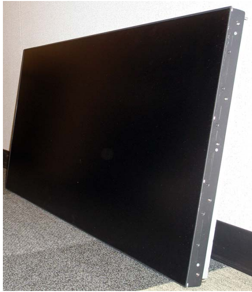
Correct position All four corners touching a solid surface Angle no more than 10° from vertical
