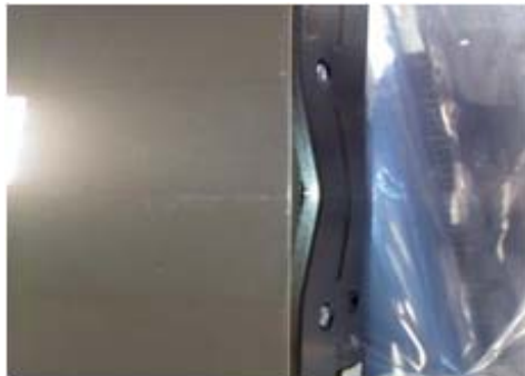
Light leakage caused by bent chassis
