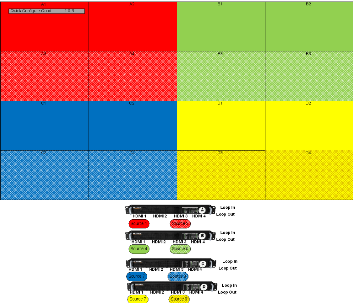
4 x 4 Matrix with two high resolution sources per Quad controller module.
