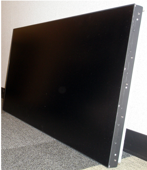
Correct position All for corners touching a solid surface Angle no more than 10° from vertical
