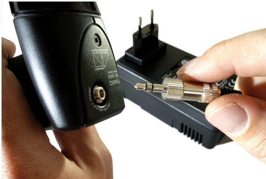
Figure 5.4: Charging the battery of the Flystick2
