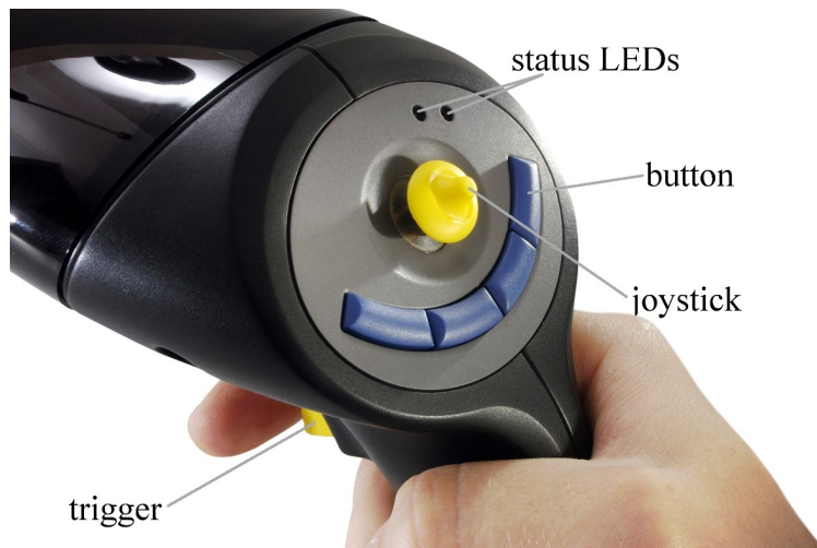
Figure 5.2: Flystick2 control elements
