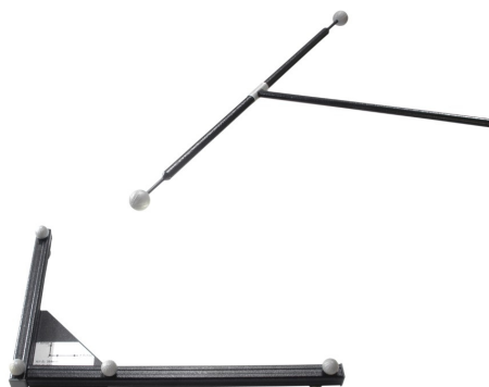
Figure 4.6: A room calibration set consisting of angle and wand
