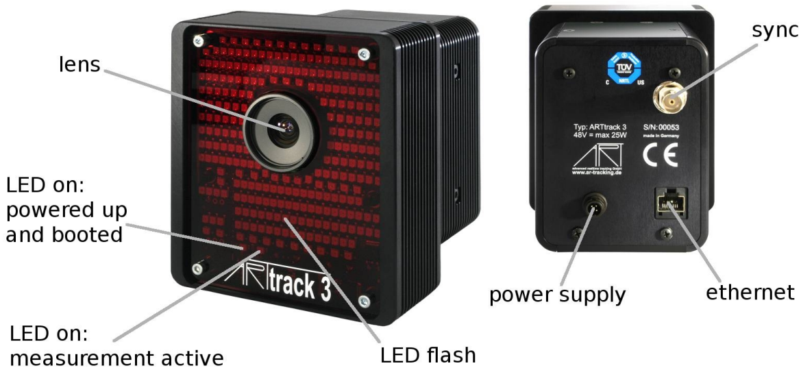
Figure 4.12: Camera ARTTRACK3 - Description of LEDs and interface connectors
