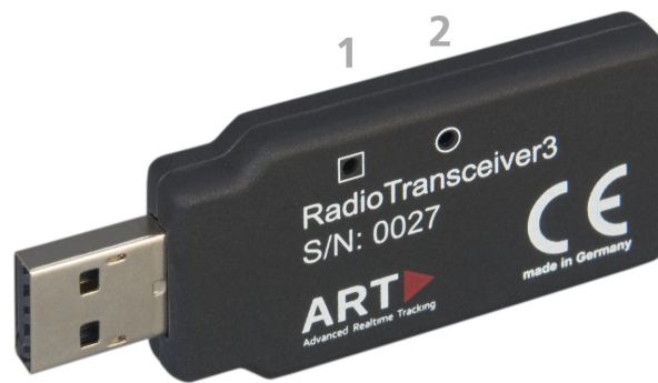
Figure 4.5: USB Radio Transceiver3 - Description of LEDs
