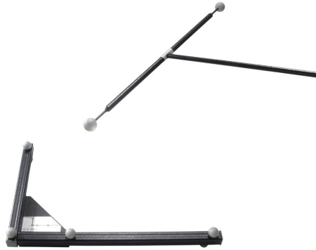
Figure 5.8: A room calibration set consisting of angle and wand
