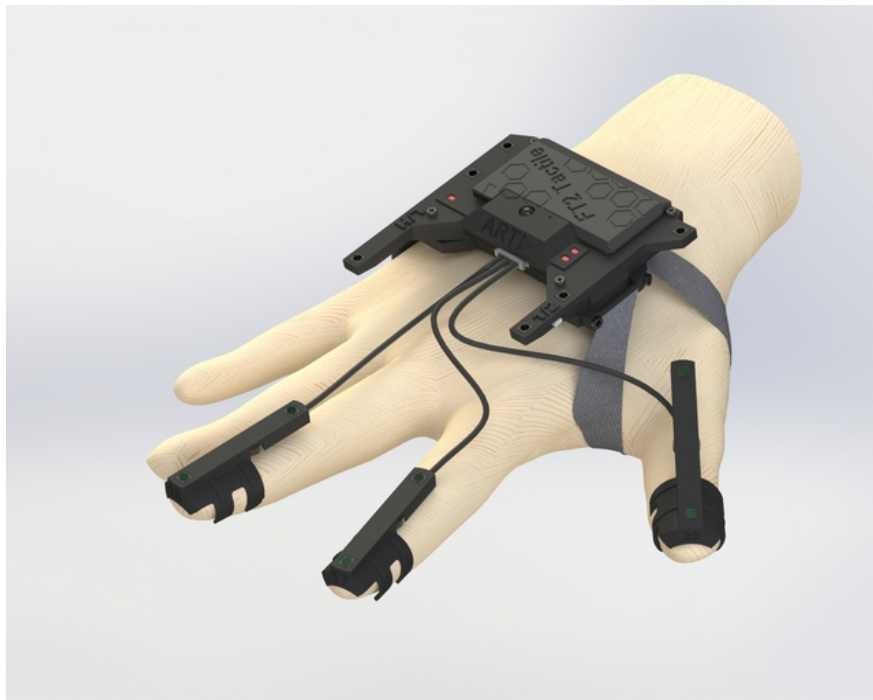
Figure 6.5: Fingertracking2 and Fingertracking2 Tactile device (shown with three active finger markers)
