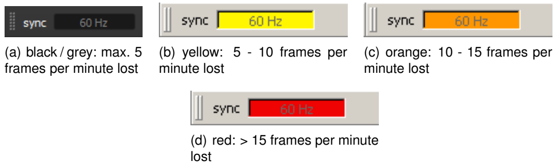
Figure 6.4: DTRACK3 Sync Status (toolbar element) - Visualization of the decrease in effective synchronization frequency
