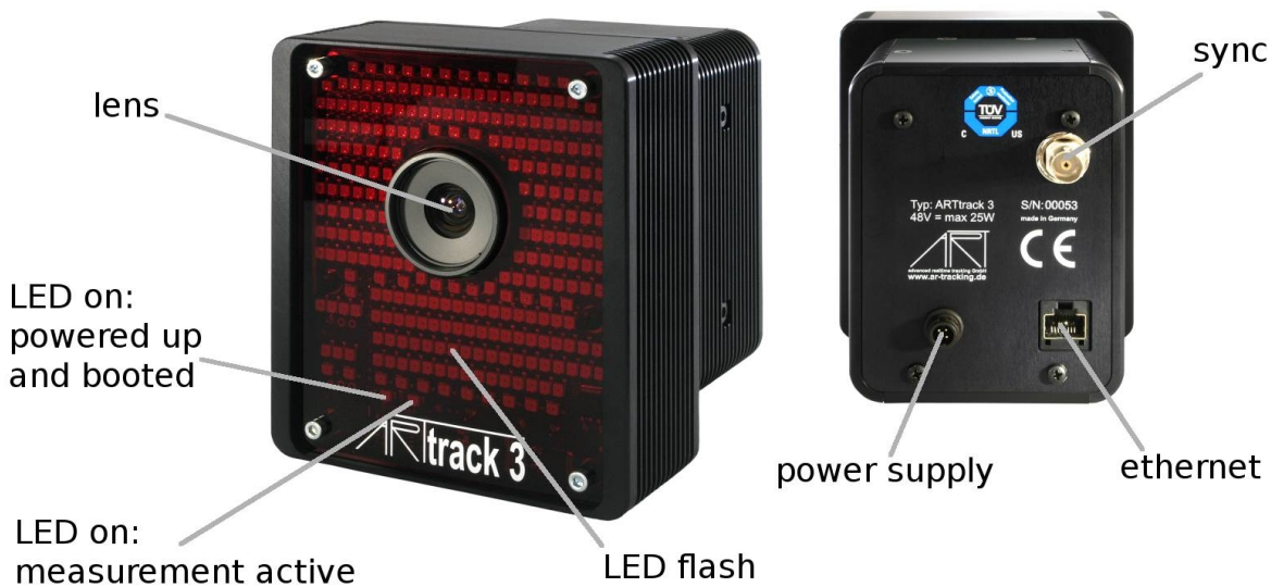
Figure 4.13: Camera ARTTRACK3 - Description of LEDs and interface connectors
