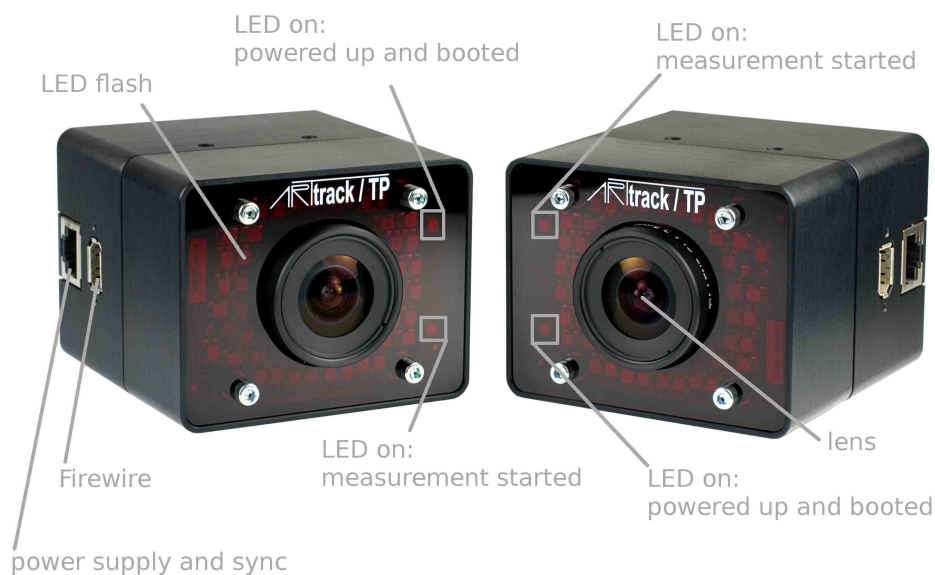
Figure 4.14: Camera TRACKPACK - Description of LEDs and interface connectors
