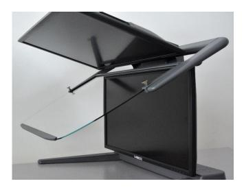
Take the Beamsplitter mirror and hold it parallel to the mirror arms. Lower the beam splitter mirror at the back so that the rear bolts slide into the grooves of the mirror holder. Then pull the mirror slightly forward until the front bolts of the mirror arm slide into the grooves of the mirror holder. Now the knurled screws (No.7) can be screwed into the provided thread in the mirror holder.
