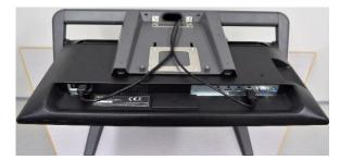
Plug the cables into the top monitor.
