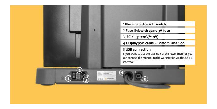
a. Connect the two Displayport cables to the graphics card of your workstation. You can find the graphics cards suitable for the 3D PluraView monitor here:
