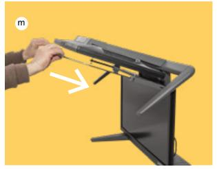
n. If you want to bring the mirror into the working position, always pull it towards you with both hands and parallel to the top screen as far as it will go and then lower it onto the mirror arm. **Never let go of the mirror prematurely. Risk of breakage!**
