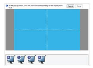
6. Select the grid position that corresponds with the physical position of the display with the blue background.
