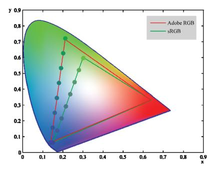
Figure 3: When the same number of colors are used to cover a larger color space, the distance between them increases which may lead to banding artifacts. To avoid this problem, the bit depth of the display device needs to be increased.
