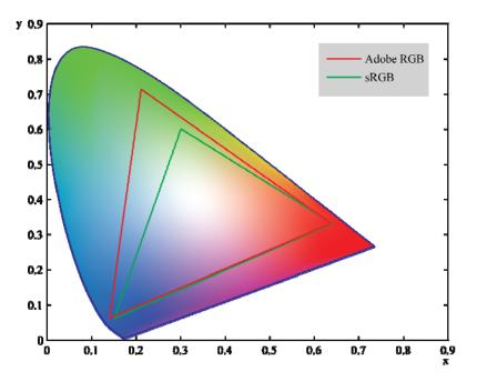
Figure 1: The 2D color gamut of the sRGB and Adobe RGB color spaces are superimposed on the CIE-xy chromaticity diagram. Note that the colors shown inside the diagram are for illustration purposes.
