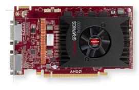
The AMD FirePro™ W5000 DVI workstation graphics can support a variety of medical imaging workflows. It can drive up to two 5MP displays independently or combined, or a drive a single 10MP display with dual input connectors as a single large desktop. Images and scans can also be viewed at a maximum resolution of 2560x2048 (in packed pixel mode), allowing professionals to see in greater detail.
