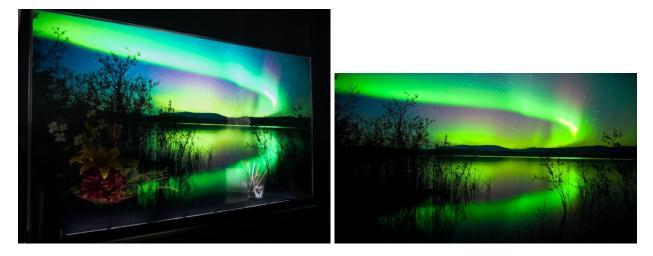
Figure 3 - Full screen image on a Planar LookThru. To the right is the image as it appears in Photoshop (note the black is opaque in the image). Note: there is a light strip in this image that is not part of the product.
