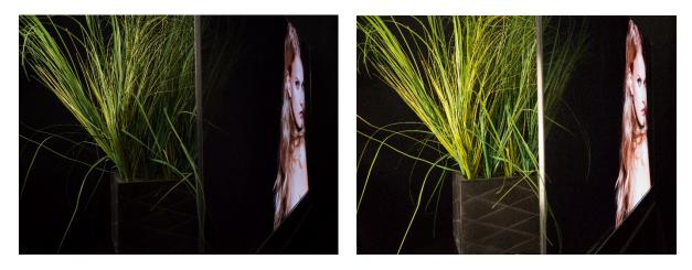
Figure 7 - Minimal lighting behind a display renders the display more opaque. Bright lighting behind the display makes the screen appear more transparent, as evidence by the grass behind visible through the display in the second image when it is not visible in the first image.
