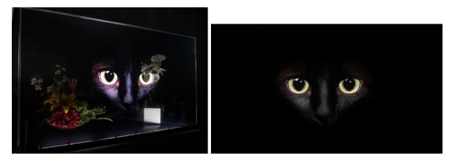
Figure 2 - The same image on the transparent display on the left and the image to the right is the picture as it appears in Adobe® PhotoShop® or a photo editing program. This mostly black image as shown on a Planar LookThru Transparent OLED Display. Note: there is a small light strip behind this display that was put there to light the floral arrangements behind the screen. That is not part of the product itself.
