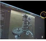
1| Media control: Via tablet PC, the display on the wall is changed to split screenmodus 2| Central remote: A cluster, consisting of four PC's in the black rack, modifying data for projection. 3| High-End Stereoscopy: The wall with DeltaGen 10.0 software. The tracking camera for interaction with the projected model, is visible at the upper right side of the wall.
