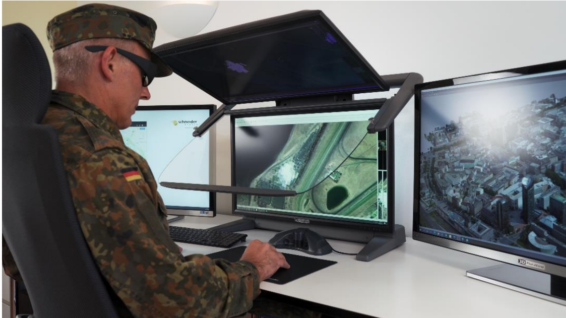
Caption: The 3D PluraView Stereo-Workspace in combination with two additional 2D displays
