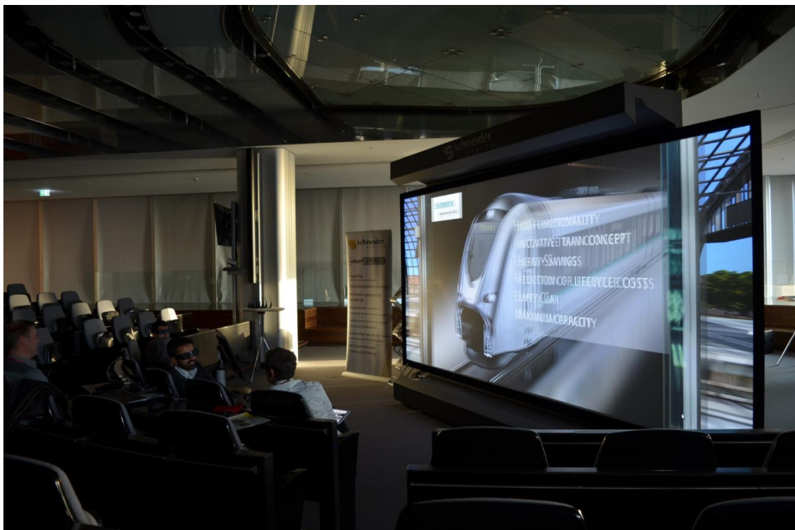
Caption: The 12 m 2 large ‚smartVR‘ PowerWall with integrated short-throw front projectors
