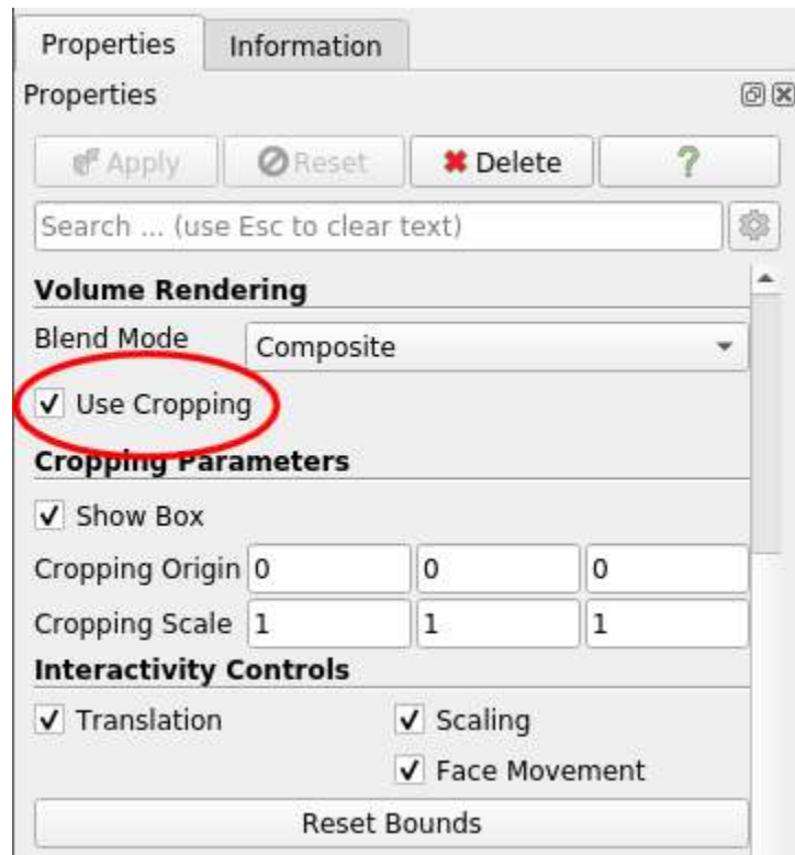
Fig. 4.10 - Cropping settings for structured grids
